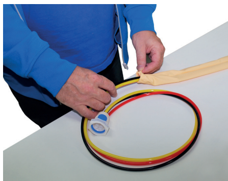
15. Pass the air tubing through its own tube sleeve. Attach the air tubing to the cell's air tube system.
