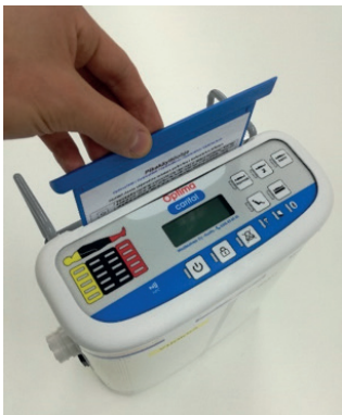
The double-sided quick guide is found on the back of the controller and is released for viewing by raising it upwards.
